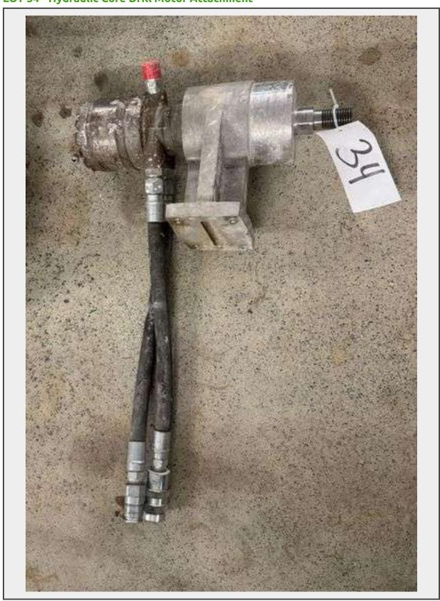
Heavy-duty hydraulic drill motor head with mounting bracket and dual hose inlets.
